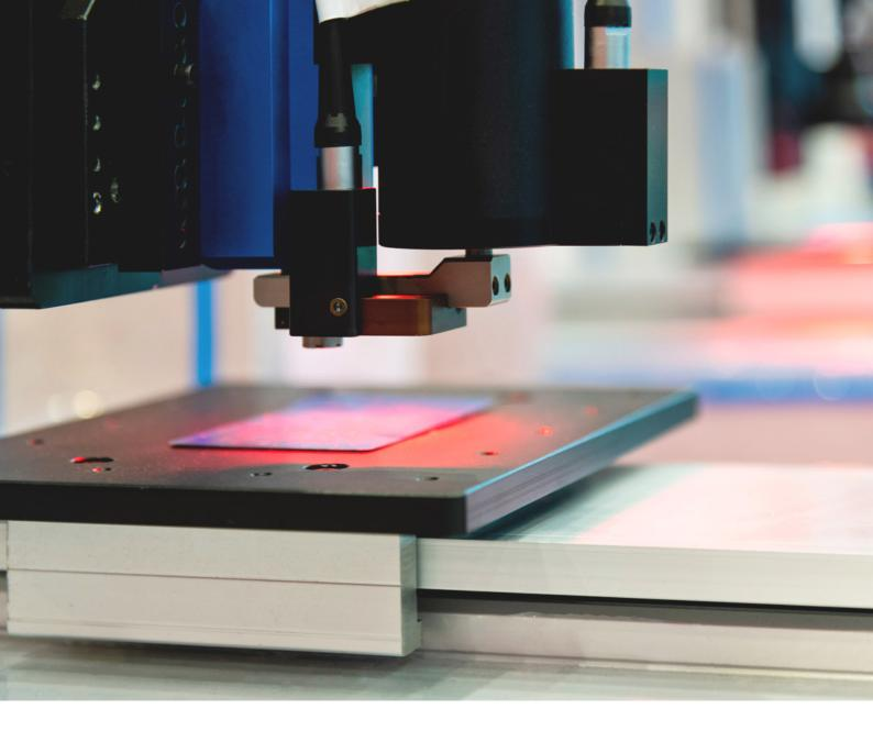
The final stage of production before a driver's licence is issued is the personalisation of the holder's data at the heart of the card, thanks to laser engraving.
