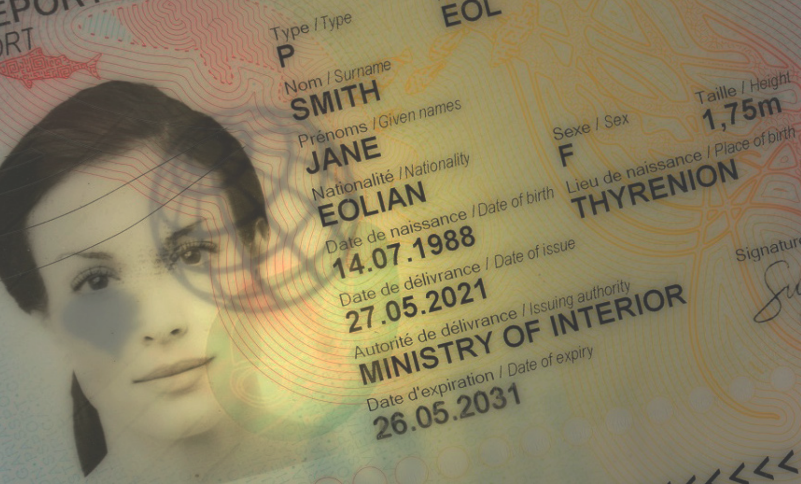
Example of a personalized aluminum “watermark” protecting the photo.
